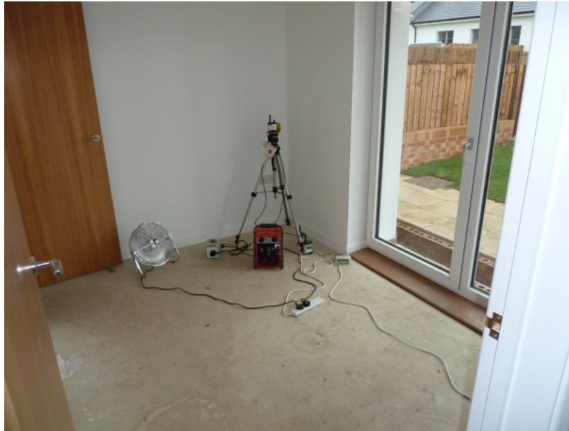
Figure 8 Main items of test equipment installed within a test dwelling.
